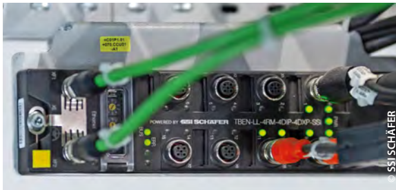
Turck has customized its TBEN-LL-4RM-4DI-4DXP I/O module for the control of CAN roller motors and for the digitalization of conveyor lines exactly to meet the demanding requirements of SSI SCHAEFER
