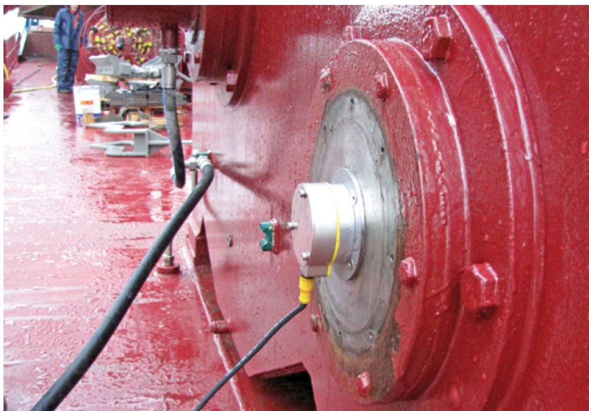
The QR24 encoder is also protected by the metal plate
